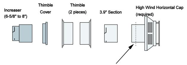
NOTE: The pipe extension (inner and outer) on the cap may need to be trimmed to fit flush against the exterior of the home (especially on 2x4 exterior walls). Make sure the cap overlaps the vent section a minimum of 2".
